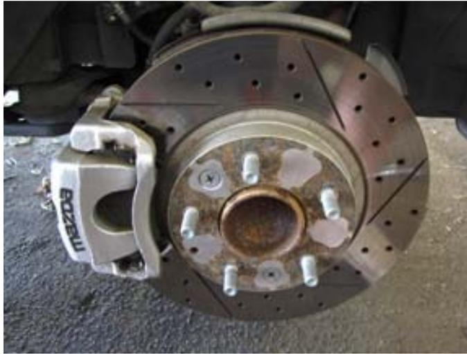
12. Swing the caliper back into position on the bracket, replace the lower caliper bolt and torque to 16-23 ft. lbs.
