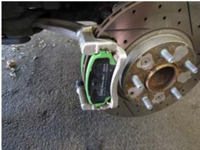
9. Place new disc pads in their proper slots in the mount bracket.
