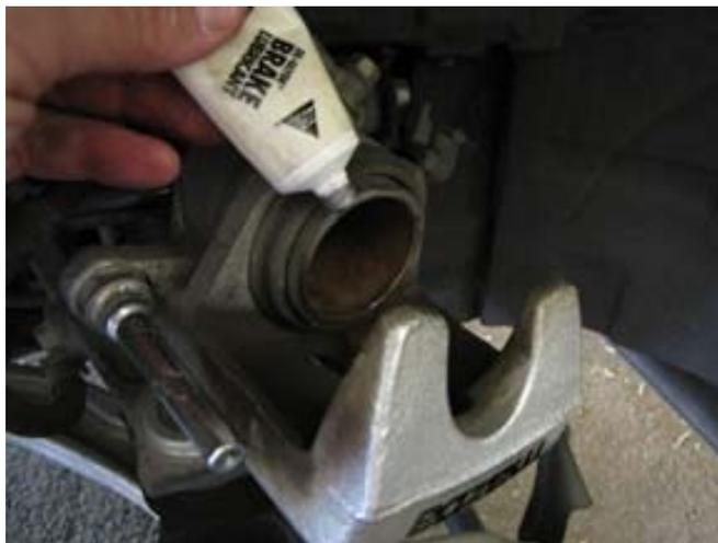
5. Lubricate the contact area of the caliper piston.
