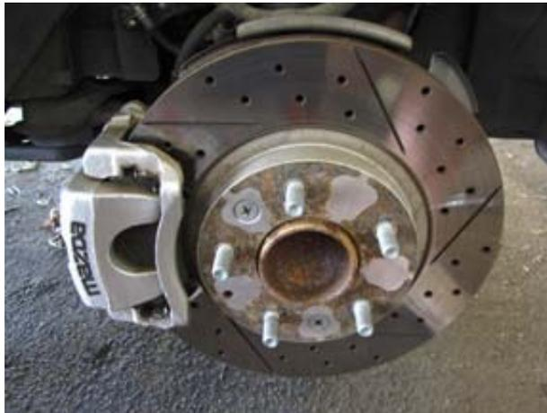
1. After placing the vehicle on jack stands remove the front wheels.
