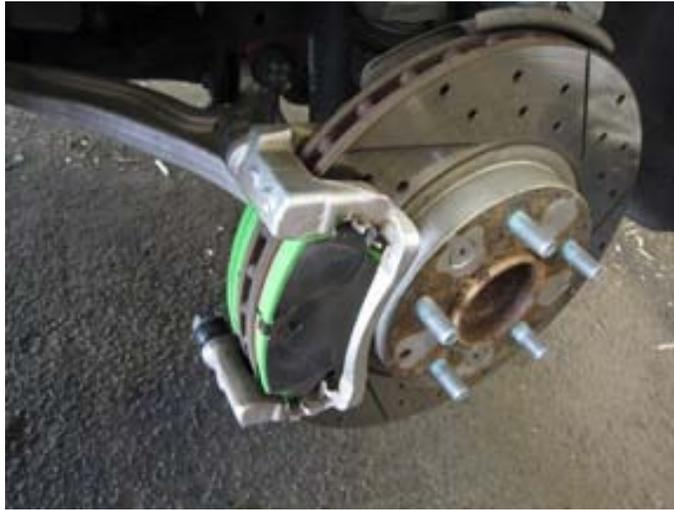
10. Put a very light coating of brake grease on the inside of the backing plates and position them on the back of the new pads.
