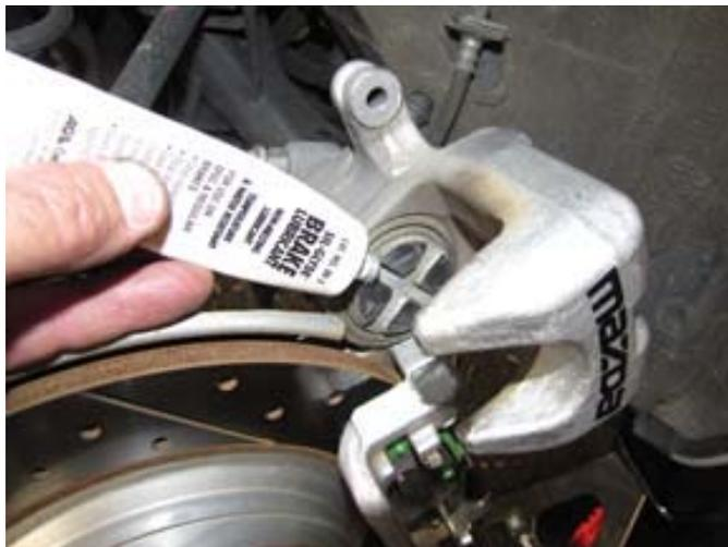
13. Lubricate the contact area of the caliper piston.
