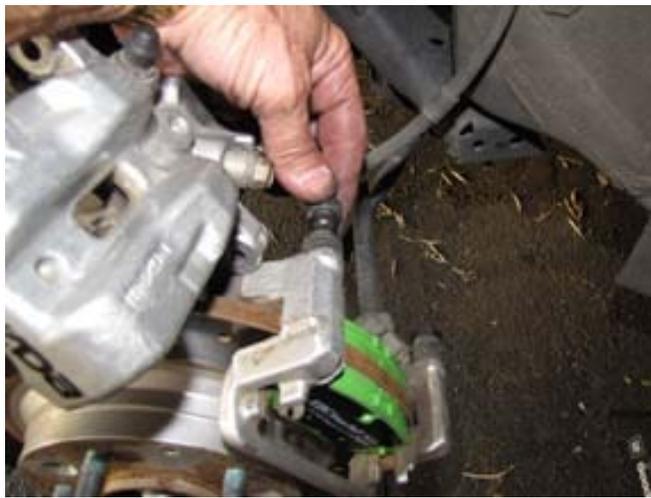
5. Replace the slider pins and make sure you get the rubber boot seated in its keeper groove.
