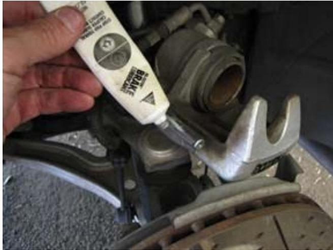
4. Lubricate upper and lower slider pins. Make sure you get the rubber boot seated in its keeper groove.
