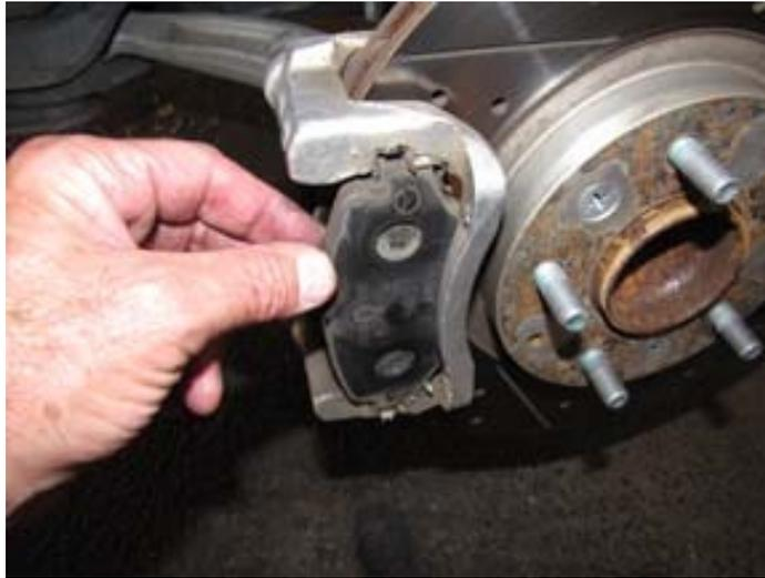
7. Remove the disc pads (inner and outer) by sliding straight out of their slots.
