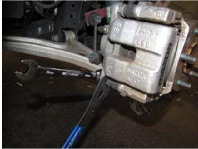
2. Using the 14 mm box end wrench and the 17 mm tappet wrench remove the lower caliper bolt.
