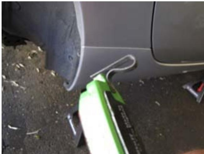
8. Pay attention to the pad with the "squealer" wear indicator clip and replace in the proper position. Mine was the inside pad, passenger side.
