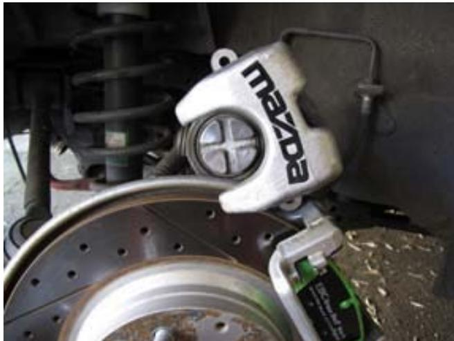
3. Remove the caliper from the mount bracket. You may have to fuss with it a bit because of a small locating pin on the inside disc pad that likes to get hung up on the caliper piston grooves.
