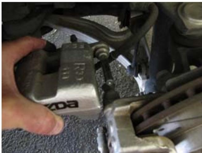
3. Swing the caliper up and ease the upper slider pin out of the mount bracket.
