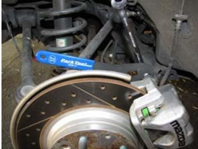
14. Place the caliper back in the mount bracket and install the caliper bolts.
