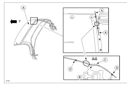
To correct the problem, a spot weld (E) has been added to the problem area, where the original spot welds are located (D), to increase the rigidity and prevent the warping.
